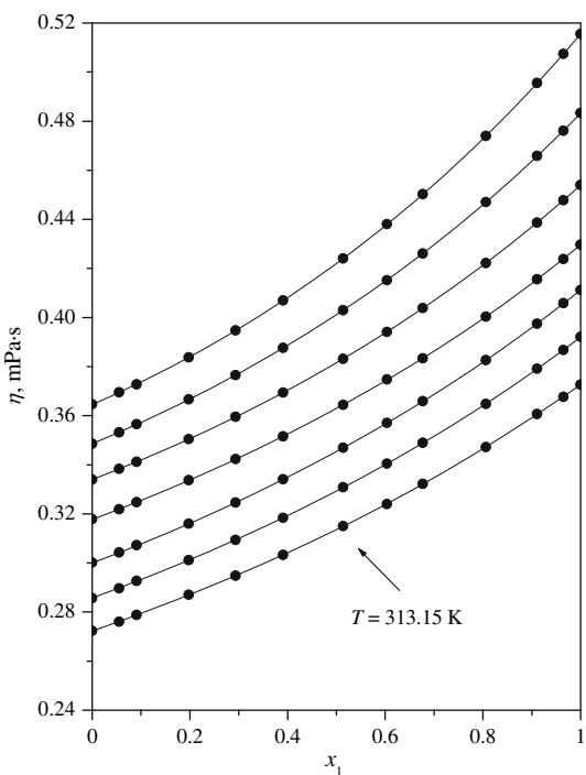
**Fig. 4** Viscosities,  $\eta$ , for 2-methyl-2-chloropropane (1) with diisopropylether (2): experimental (●); correlated values (—)
