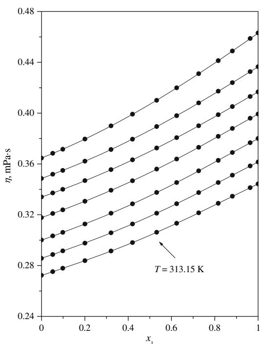
**Fig. 3** Viscosities,  $\eta$ , for 2-methyl-1-chloropropane (1) with diisopropylether (2): experimental (●); correlated values (—)
